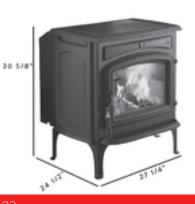
Heating Capacity Up to 2,600 sq. ft. 83,000 BTU/hr Max Heat Output Up to 18" front to back Log Size Emissions 3.50 Grams/hr Burn Time Up to 10 hrs 2.95 ft<sup>3</sup> Firebox Size Weight 475 lbs Clearances Top Vent Rear 10" w/FCHS Side 14" Corner 12" Clearances with rear heatshield & double wall chimney connector Rear 6" Side 14" Corner 12" Height to top of flue Top (30 5/8") Rear (30") Minimum Hearth Dimensions (W x D) 33" x 40 3/4"
