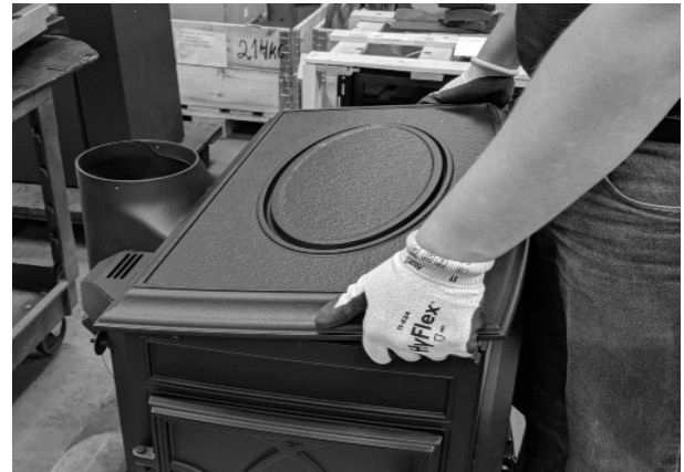
Fig. 21. Remove the top plate from stove.
