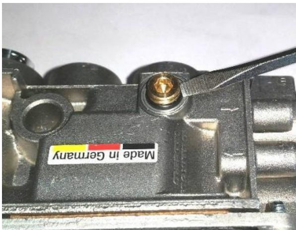
Figure 22 – Low Flow Orifice Removal – O-ring
