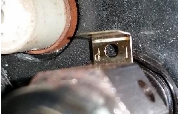
Figure 28 – Pilot in LP (LP text visible to rear of Pilot Tower)
