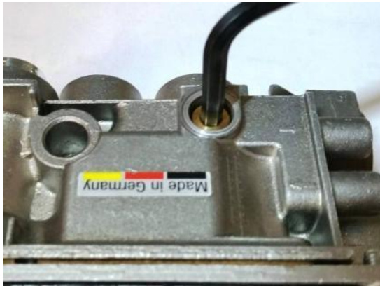
Figure 21 – Low Flow Orifice Removal
