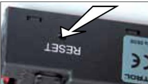
Figure 41 – Receiver Reset Button Location
