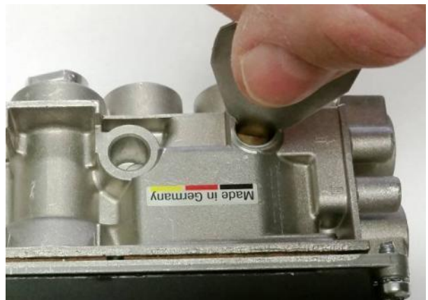
Figure 25 – Tighten LP Low Flow Orifice
