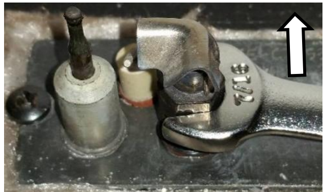
Figure 26 – Pilot in NG (Pilot Gate forward)
