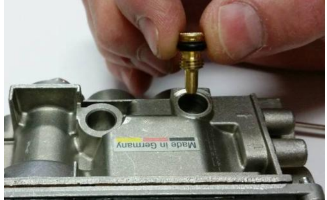
Figure 23 – NG Low Flow Screw Removal
