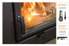
**3)** Allow the fire to build, adding kindling until the fire has a hold. After 5-10 minutes add medium sized logs, after a further 5-10 minutes close the door.
