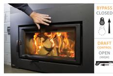
**4)** Once the fire becomes established add large logs to the firebox until it is fully loaded. Typically, after 20-30 minutes you should be able to **close the bypass damper** as temperatures will have reached the "active" zone (beyond 500° F, 260° C).
