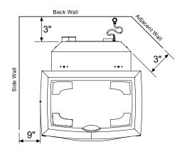
NOTE: Clearances are measured from the high efficiency adaptor, if installed. All product specifications are subject to change without notice. Before installing refer to the relevant product manual for full and up to date information.
