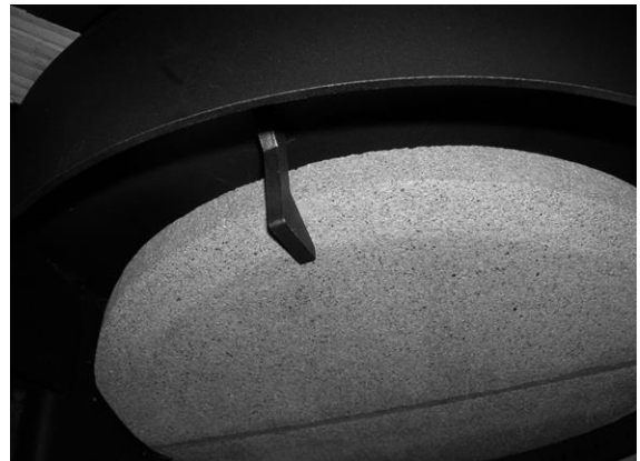
Figure 8 - Removing/Replacing the Baffle for Inspection
