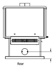
With pedestal from base of unit to centerline 5-1/2" (138mm)
