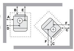
**NOTE:** This clearance is also required for air space between the appliance and wall/ceiling. Clearances to combustibles are for the safety of the property. To avoid overheating and damaging the appliance these clearances should be maintained for non-combustibles also.
