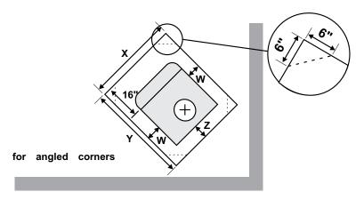
\*\*NOTE: In Canada, floor protection must extend 18" (457mm) to the front.
