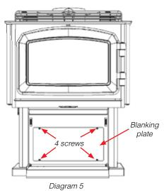
9. Place unit into position and install the mandatory outside air kit. See «Mobile Home installation» section in this manual.
