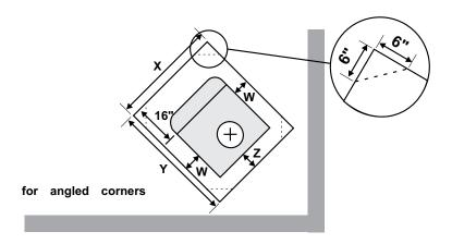
\*\*NOTE: In Canada, floor protection must extend 18" (450mm) to the front and 8" (203mm) to back of the stove.
