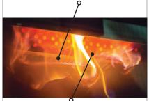
Bypass closed; located inside firebox (top front)
