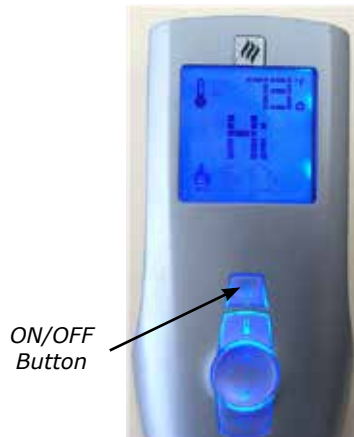
Diagram 1 Remote shown in Manual Mode on Hi
